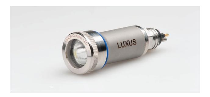
The LUXUS Compact LED light is ideal for diving applications. The LED has an output of 440 or 780 lumen and is available with different reflectors. The LUXUS Compact LED is a wet and dry light and can be used from 4,000 metres depth up to the deck without needing to be switched off. The electronics have an auto resetting thermal protection switch that protects the LED and LED driver from high temperatures.
