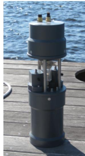
EcoLAB adapts established wet chemical methods to an *in-situ* chemical analyzer. Precise volumes of sample, on-board standard and reagents connected to a rotary valve are mixed by a syringe pump and reacted solutions are analyzed in colorimeters. In essence, the EcoLAB is a submersible “chemistry robot”.
