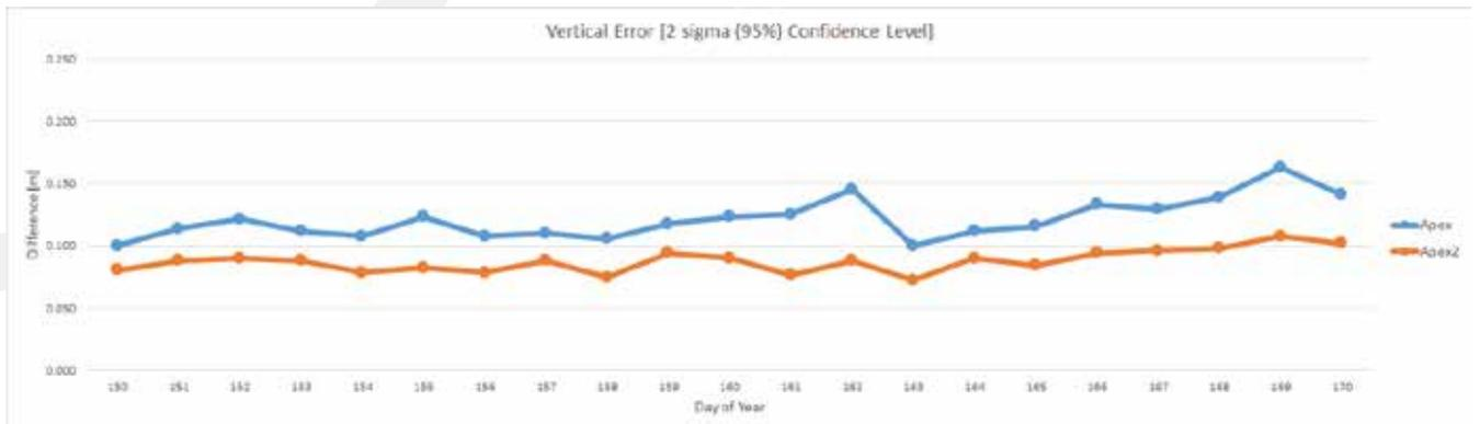
Above: horizontal and vertical position errors in VERIPOS Apex solution at a monitor site in Aberdeen.
